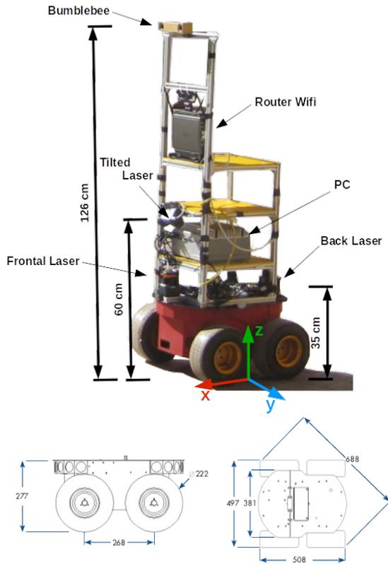
Fig. 1. Top: General platform configuration: Location of the lasers and the bumblebee camera, plus others components. The origin frame is also indicated. Bottom: Dimensions of the platform. Measurements are in *mm*. Source: <http://www.mobilerobots.com/ResearchRobots/P3AT.aspx>
