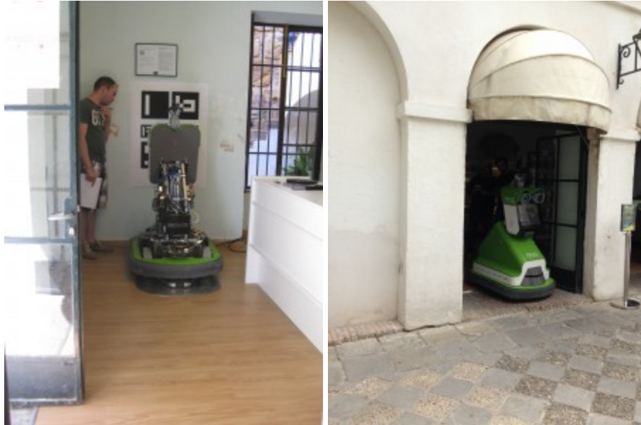
Fig. 2.3. Left: FROG robot on its stainless steel docking station, surrounded by wood laminate floor. Right: FROG making the transition from wood laminate over a brick doorstep onto flagstone/cobble chequered courtyard.
