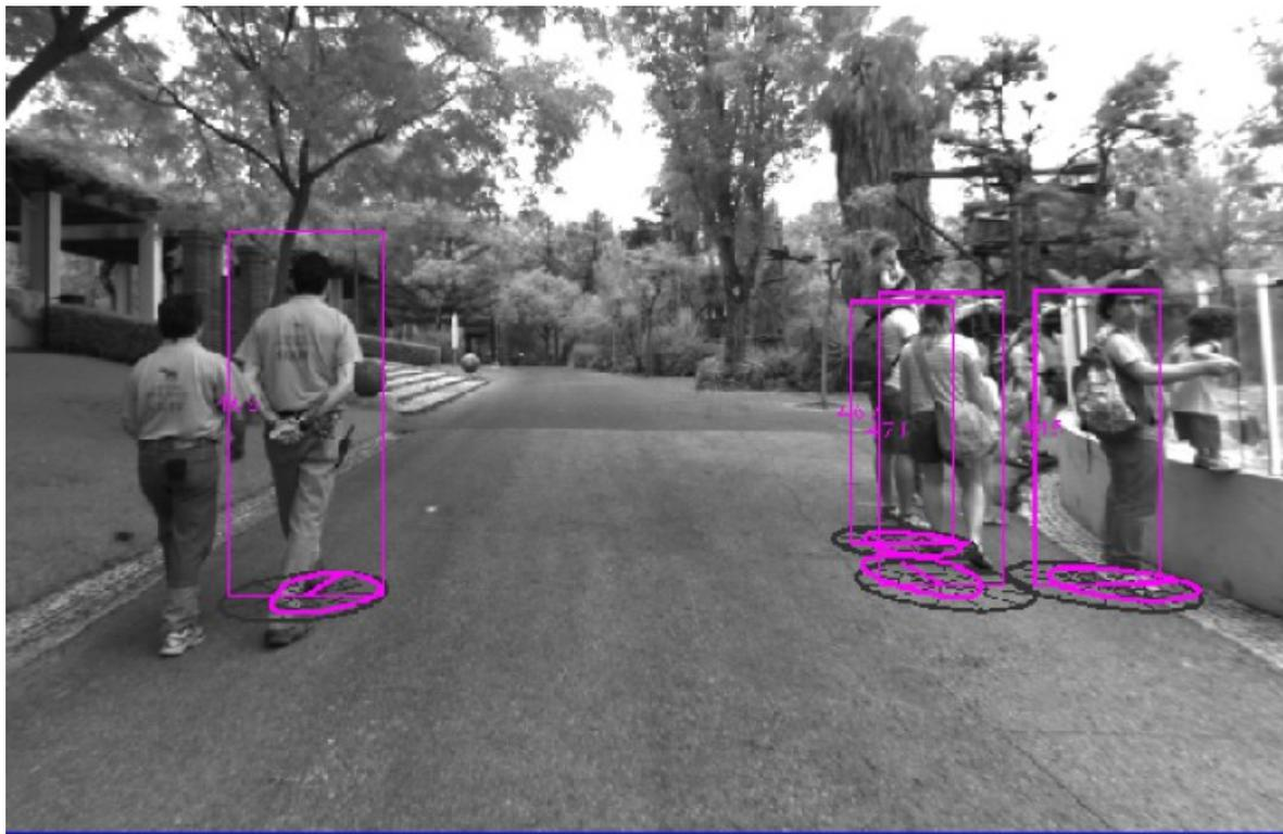
Figure 3. Person detection and body orientation estimation based on stereo cameras detection.
