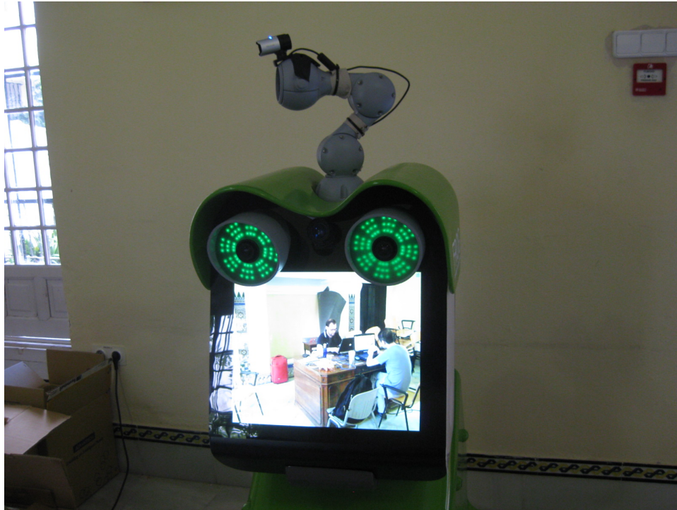
Testing the webcam temporarily mounted on the antenna
