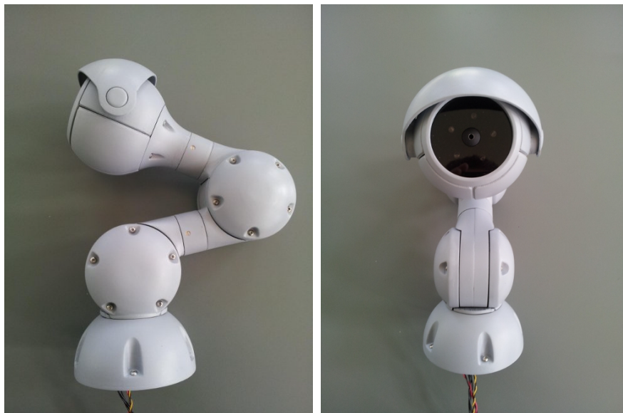
Antenna with laser pointer and LEDs
