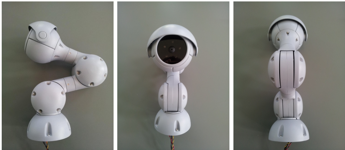
Figure 23: 3DOF arm with laser pointer
